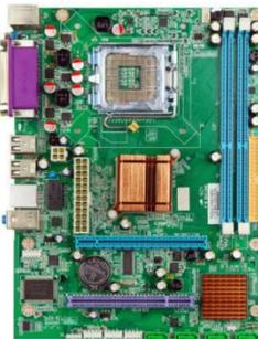
The motherboard is the backbone that ties the computer's components together at one spot and allows them to talk to each other. Without it, none of the computer pieces, such as the CPU, GPU, or hard drive, could interact. Total motherboard functionality is necessary for a computer to work well.
