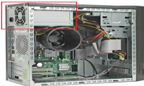
A power supply unit (PSU) converts mains ac to low-voltage regulated dc power for the internal components of a computer.
