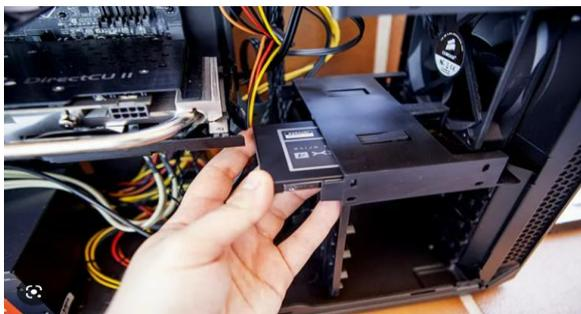
Solid-state drives (SSD) are the most common storage drives today. SSD are smaller and faster than hard disk drives.
